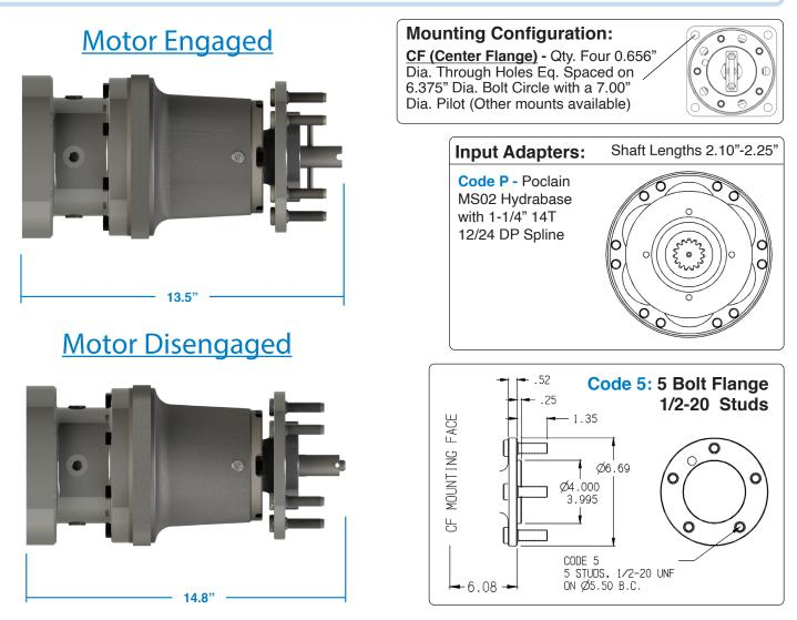
Model 12CF5-41-1 Shown Above with Code 5 Flanged Output Shaft and Code 4 SAE A Input with 1-1/4" 14T Spline
