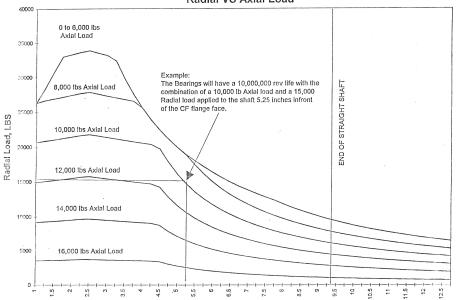
Load Position, inches from CF Mounting Flange Face
